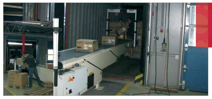
A manual job is made easier. Unloading containers is a strenuous, manual job that can result in repetetive strain injuries and/or a high level of absence owing to sickness. MUSIK MEYER decided to reduce the risks involved, and indeed the cost of having a reduced workforce due to sickness, by providing the operators emptying containers with a lifting aid.
